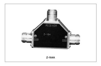
The Z-164A/B is used as a matching pad for applying the mixed output of two signal generators to the input terminal of a receiver for measuring two-signal characteristics (such as the blocking and intermodulation characteristic) of the receiver.
